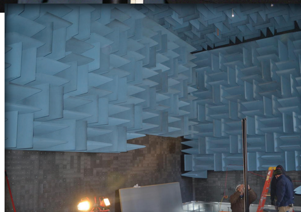
▲ EECS seniors Luke Ezell and Jalashree Mehta prepare the anechoic chamber for antenna measurements.
