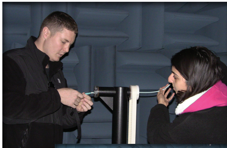
▲ EECS seniors Luke Ezell and Jalashree Mehta prepare the anechoic chamber for antenna measurements.
