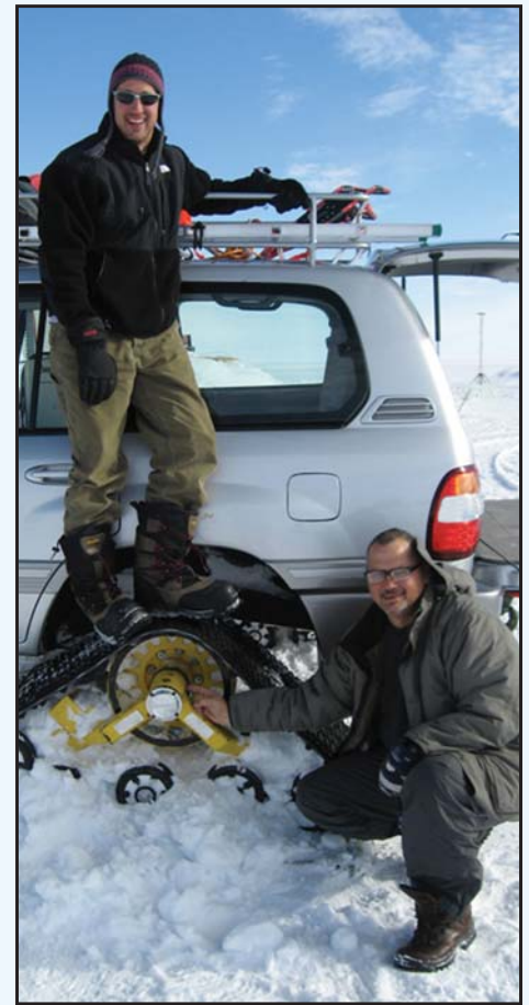
EECS Assistant Professor Carl Leuschen (standing) and CReSIS technician Dennis Sundermeyer show off the makeshift solution devised after the bearings broke on the vehicle towing the radar sled.
